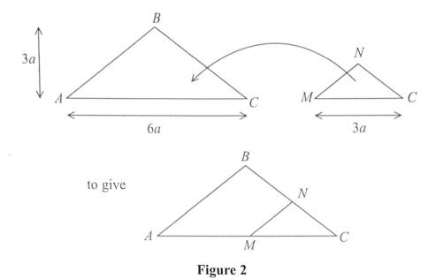
The uniform lamina ABC is an isosceles triangle with AB = BC, AC = 6a and the distance from B to AC is 3a.
