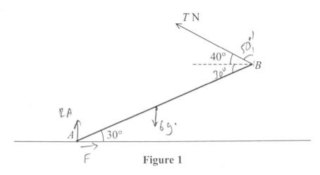
A uniform rod AB, of mass 6 kg and length 1.6 m, rests with its end A on rough horizontal ground. The rod is held in equilibrium at 30° to the horizontal by a light string attached to the rod at B. The string is at 40° to the horizontal and lies in the same vertical plane as the rod, as shown in Figure 1. The tension in the string is T newtons. The coefficient of friction between the ground and the rod is  $\mu$ .
